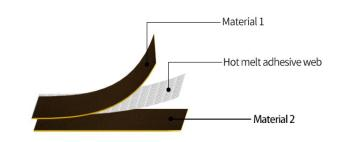
Example: Plan view of double-layer material bonding:
