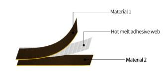
Example: Plan view of double-layer material bonding:
