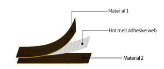
Example: Plan view of double-layer material bonding:
