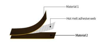
Example: Plan view of double-layer material bonding:
